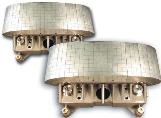
The picture shows two prototype outer poloidal limiter tile assemblies which stack together to hide the remote handling bolts and carriers thereby maximising the power handling. Tile surfaces are segmented to relieve the stresses caused by thermal expansion and to reduce electromagnetic forces.
